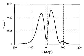
FIGURE 12. Comparison of root-mean-square density of scattered wave. —, Direct simulation results;  $\cdots$ , computed from (18) with  $\hat{S}$  measured from computations. (M = 0.125).
