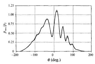
FIGURE 3. Comparison of root-mean-square pressure level of scattered wave, normalized by the amplitude of the incident waves, between simulations on different-sized domains: ——, Domain 1; ———, Domain 2. See figure 2 for domain sizes.
