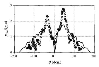
FIGURE 22. Comparison of predicted scattering amplitude with experimentally measured result (Horne 1983): ——, analysis,  $\bigcirc$ , experiment.
