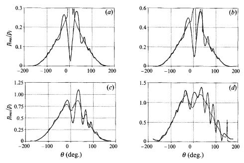
FIGURE 19. Root-mean-square pressure level of scattered wave at  $r = 2.5\lambda$ . (a)  $\epsilon = 0.14$ , (b)  $\epsilon = 0.27$ , (c)  $\epsilon = 0.55$ , (d)  $\epsilon = 1.1$ . —, Navier-Stokes solutions with  $\tilde{r}_0 = \frac{1}{2}\pi$ ; ——, high-frequency approximation.
