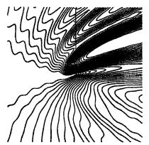
FIGURE 4. Iso-contours of the root-mean-square pressure level of the scattered wave, normalized by the amplitude of incident wave. Contour levels: Minimum = 0.08; Maximum = 1.12; Increment = 0.04. ( $\epsilon = 0.27$ ,  $\lambda/L = 4$ , M = 0.125).
