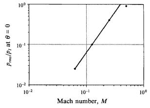
FIGURE 9. Scattering in the forward direction versus Mach number: •, data from computations; —, line with slope 2.
