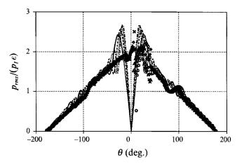
FIGURE 21. High-frequency scattering amplitude compared with long-wavelength analytical solution. Lines are from long-wavelength analysis,  $\tilde{r}_0 = \frac{1}{2}\pi$ : —,  $r/\lambda = 3$ ; ——,  $r/\lambda = 4.5$ ; ……,  $r/\lambda = 6.0$ ; ——,  $r/\lambda = 7.5$ . Symbols are from high-frequency approximation with  $\epsilon = 0.30$ :  $\bigcirc$ ,  $r/\lambda = 3$ ;  $\times$ ,  $r/\lambda = 4.5$ ;  $\diamondsuit$ ,  $r/\lambda = 6.0$ ;  $\triangle$ ,  $r/\lambda = 7.5$ .  $x_0 = 200$ .
