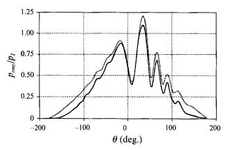
FIGURE 10. Comparison of root-mean-square pressure level of scattered wave between simulations on different sized domains. e = 0.55,  $\lambda/L = 4$  (M = 0.25): ——, Domain 1; · · · · · · , Domain 3. See figure 2 for domain sizes.
