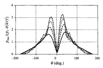
FIGURE 7. Root-mean-square pressure level normalized by right-hand side of (8);  $\epsilon = 0.14$ ,  $\lambda/L = 4$  (M = 0.0625): ---,  $r/\lambda = 1$ ; ----,  $r/\lambda = 1.5$ ;  $\cdots \cdots$ ,  $r/\lambda = 2$ ; ----,  $r/\lambda = 2.5$ .
