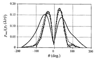
FIGURE 11. Root-mean-square pressure level of scattered waves, normalized by amplitude of incident wave and  $(\lambda/r)^{\frac{1}{2}}$ . M = 0.125,  $\lambda/L = 4$ : —,  $r/\lambda = 0.5$ ; —,  $r/\lambda = 1.0$ ; …,  $r/\lambda = 1.5$ ; —,  $r/\lambda = 2.0$ ; —,  $r/\lambda = 2.0$ ; —,  $r/\lambda = 2.5$ .
