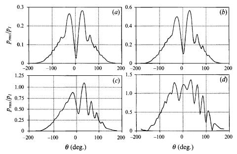
FIGURE 5. Root-mean-square pressure level of the scattered wave at  $r = 2.5\lambda$ . (a)  $\epsilon = 0.14$  (M = 0.0625); (b)  $\epsilon = 0.27$  (M = 0.125); (c)  $\epsilon = 0.55$  (M = 0.25); (d)  $\epsilon = 1.1$  (M = 0.5).
