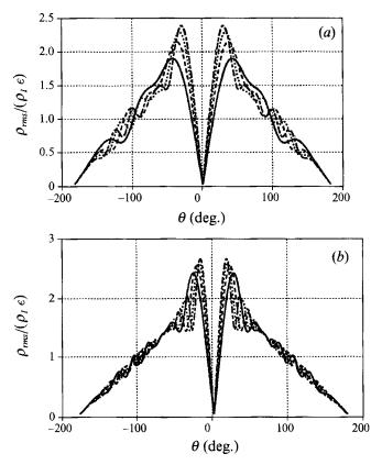
FIGURE 14. Root-mean-square density level from analysis, (44). (a)  $\lambda/L = 4$ : —,  $r/\lambda = 1$ ; ——,  $r/\lambda = 1.5$ ; …,  $r/\lambda = 2$ ; ——,  $r/\lambda = 2.5$ . (b)  $\lambda/L = 4$ : —,  $r/\lambda = 3$ ; ——,  $r/\lambda = 4.5$ ; …,  $r/\lambda = 6.0$ ; ——,  $r/\lambda = 7.5$ .
