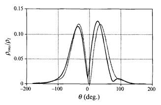
FIGURE 13. Comparison of root-mean-square density of scattered wave. —, Computed from (16) with  $\hat{S}$  measured from computations; ..., computed with analytical source term given by (19). (M = 0.125).
